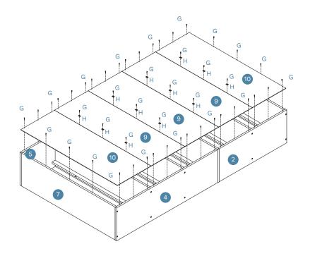
Attach assembled furniture together as shown and secure with 2 x screws (E) and 4 x cam locks (B). Tighten with a screwdriver.
