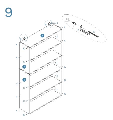
Once assembled lift furniture into place, do not drag. Use a drill to create a small hole lining up with the top of the 2 x wall anchors (F). Fasten to the wall using 2 x wall plugs (I) and 2 x screws (E). Attach 20 x screw covers (K) to assembled frame as shown. Ensure unit is balanced and steady before use. You're done, enjoy!
