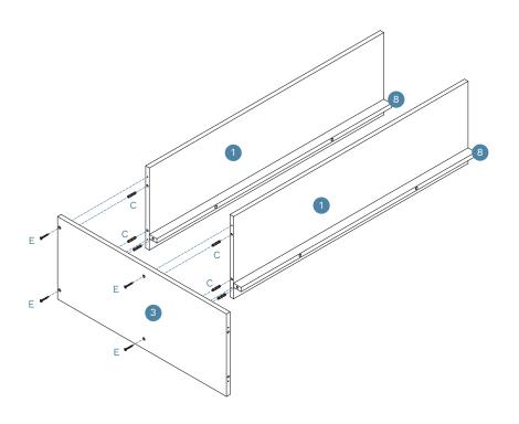
Attach panel (4) to assembled frame as shown and secure with 9 x short dowels (C) and 6 x screws (E). Tighten with a screwdriver.
