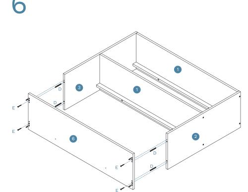
Attach panel (6) to assembled frame as shown and secure with 4 x long dowels (D) and 4 x screws (E). Tighten with a screwdriver.
